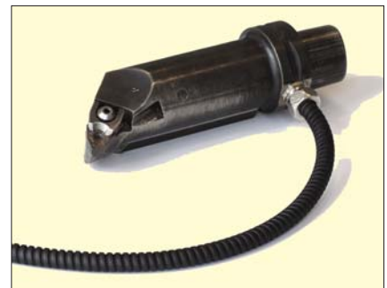
Figure 5. An Acticut tool holder with embedded sensors and actuators.
