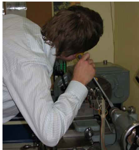
Figure 7. Example of a classical approach using a screw driver to monitor the "cutting parameters" from the machine while turning.
